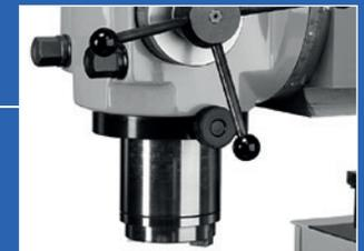
Fine feed for BSF drilling spindle
